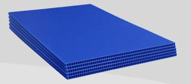
A 1m x 2m, semi flexible, polypropylene based board, double layered with 5mm integrated perpendicular support spacers at 4mm intervals, to be applied as a protection to the waterproof membrane
